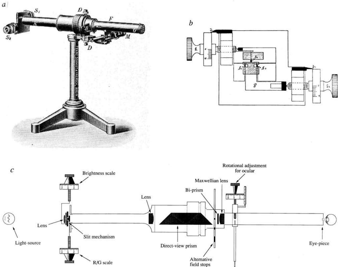
FIG. 2 a, Nagel anomaloscope Model II in its original form<sup>4</sup>. The eyepiece is on the right of the instrument and the slit mechanism on the left. The difference between Models I and II is that Model II has a facility to change the angle of the ocular, and thus the three primaries selected for the equation. b, Detail of the slit mechanism. Movement of the tongue (P) between the two sides of the slit increases either the red or the green
